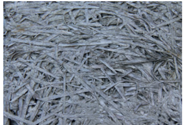
wood fibre cement boards, used as ceiling panels (2016)
