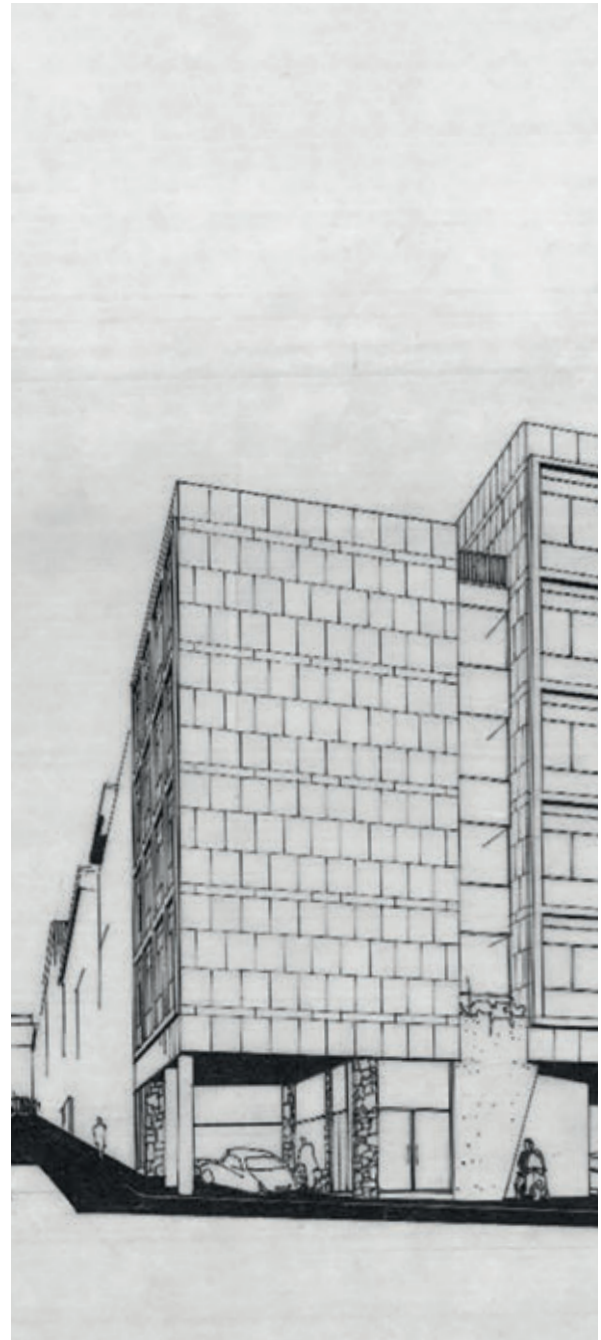
precast concrete façade panels: current condition (left) and original design (right). The 1956 sketch also shows the ‘open’ corner for cars.
